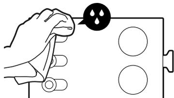
For thorough maintenance, we suggest you use the Lelit cloth (Cleaning Kit code PLA9101 – not included), which will help you clean the nozzles and the spaces between the gaskets more effectively, removing stains and coffee residues from even the smallest cracks.
