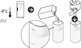
**3** Place a Cappuccino cup or a Latte Macchiato glass under the coffee outlet and adjust milk spout position by rotating it up to the centre of the cup. Turn the milk froth regulator knob to the
