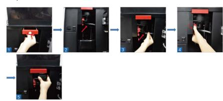
Step 2: Take off the cover of mixer, and remove the mixer impeller, then clean it by water.
