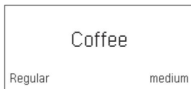
**i** You can change the cup size and coffee strength by touching [ ml ] and [ Ø ]. If you select Ground coffee, follow the procedure described under "Preparation using ground coffee".
