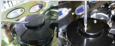
Loosen the bleed screws one at a time to allow air to escape until water flows from below the screw head. Tighten the screw to stop the water from flowing. Over tightening can cause damage to the sealing washer and the group cover. Repeat this procedure on all groups.
