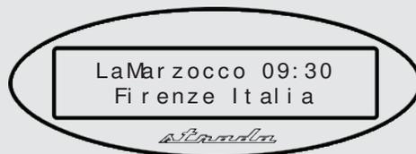
The digital display is a backlit display capable of displaying 2 lines of 16 characters. The display enables the operator to interact with the espresso machine to visibly change parameter values. The display also provides valuable information to the operator. There are several warnings that can be displayed to alert the operator of an unusual condition or a fault. Additionally, simple messages are displayed alerting the operator that an action has been started or that a process needs to begin.
