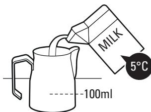
Fresh whole milk provides a smoother, creamier and tastier froth. Milk will not froth at over 65°C, so cold milk from the fridge should be used to allow more time for it to froth. The best jug, on the other hand, is one made of stainless steel, provided with a spout, such as Lelit models (codes PLA301L - PLA301M - PLA301S - not included). The level of milk should never exceed half the volume of the jug.
