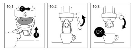
Choose your coffee filter, insert it into the portafilter (G) and fill it with the adequate quantity of ground coffee. Use the tamper (D) to press the coffee powder in the portafilter (G). Fix the portafilter (G) into the brewing group (13) and make sure the handle is aligned with padlock symbol present on the group (Pic 10.1).
