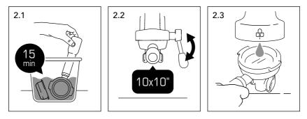
**Backflushing.** Insert the blind filter (C) into the portafilter and pour 1 bag of detergent powder (F or PLA9201) into the filter. Insert the portafilter (G) in the group (13) and lift the lever (14) for 10 seconds. Stop the function and wait for 10 seconds. Repeat the procedure 10 times (Pic 2.2).
