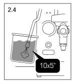
**Steam wand cleaning.** Fill a jug with 500 ml of cold water, add the content of 1 bottle of detergent liquid (F or PLA9203) and immerse the steam wand (7) in this solution.
