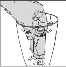
Immerse the INTENZA+ water filter vertically (with the opening pointing up) in cold water and gently press its sides to let any air bubbles out.
