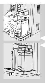
**3** Push the carafe towards the bottom while rotating it at the same time until it is locked onto the (external) drip tray (E).
