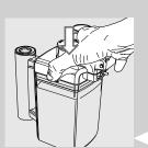
2 Refit the lid and insert the milk carafe into the machine.
