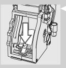
**9** Gently pull down the lever until it is in contact with the brew group base and the two reference marks on the side of the brew group match.
