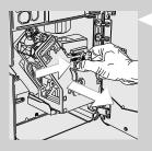
**3** To remove the brew group, press the «PUSH» button and pull it by the handle.
