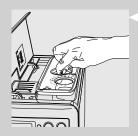
8 Lift the coffee bean hopper lid and remove the inner lid.
