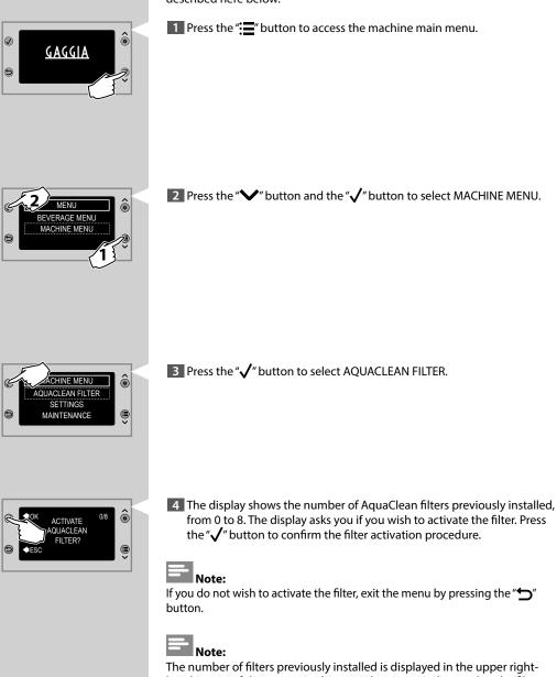
hand corner of the screen. In this case, the screen indicates that the filter being installed is the first one. This number is very important: after the
