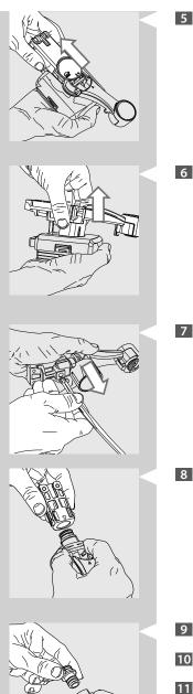
5 Remove the connector which comes into contact with the machine.
