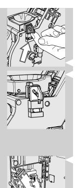
Make sure that the hook which locks the brew group is in the correct position. If it is still in the downward position, push it upward until it locks correctly into place.
