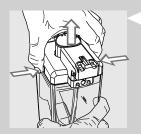
2 Press the release buttons to remove the lid.
