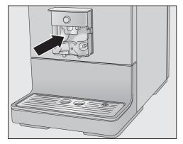
Clean the surfaces of the central spout and the dispensing spouts with a damp cloth. Clean any blockages in the milk pipework under running water with the special brush supplied:
