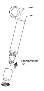
• The steam wand can be left immersed in the milk jug filled with water when not in use to reduce the risk of blockages.
