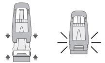
• To install the assembled filter holder into the water tank, align the base of the filter holder with the adapter inside the water tank. Push down to lock into place.
