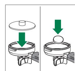
Insert the blind filter disk and add the detergent supplied or an equivalent. Lock the portafilter
