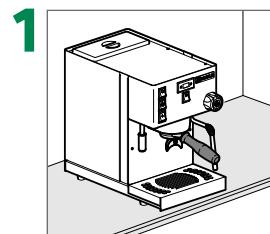
1 Put machine on a level and stable surface
