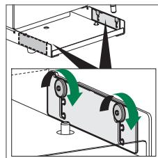
Secure the locking nuts and position the gliders
