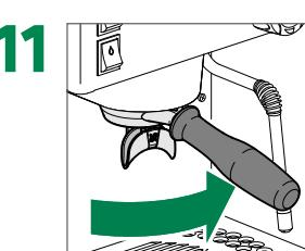
Insert portafilter into group head, empty the drip tray and relocate the grid
