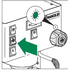
Press the steam button; when the boiler is ready, the LED will light up and remain on
