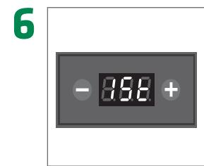
6 1St (1st Start Up): Wait for water loading to be completed in the coffee and steam boilers
