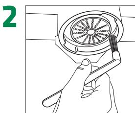
Clean the portafilter gasket using the supplied brush
