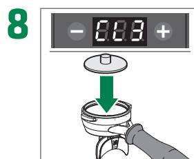
When the display shows CL3, remove the portafilter and insert the blind filter disk once again
