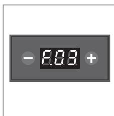
To empty the coffee boiler, place a container under the coffee outlet, choose **F.03** from the menu and confirm
