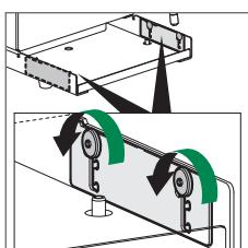
Loosen the locking nuts
