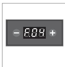
To empty the steam boiler, place a container under the water spout, choose **F.04** from the menu and confirm
