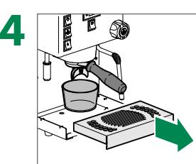
Remove the grid and place a container to collect rinsing water
