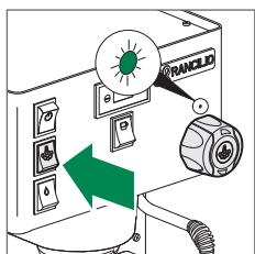
Press the steam button; when the boiler is ready, the LED will light up and remain on
