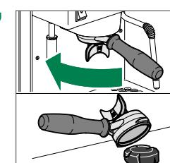
7 Remove the portafilter to empty and clean it, perform a flush and then reattach it
