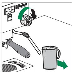
After the desired brewing, close the tap and remove the pot. Clean the wand with a damp cloth
