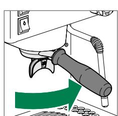
4 Lock the portafilter into the group head and put cup(s) under coffee outlet
