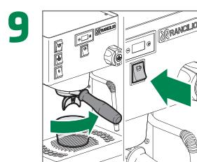
Lock the portafilter back in place and press the coffee button to continue the washing cycle
