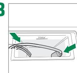
3 Ensure that the tubes are inserted in the reservoir and that the vacuum trap is fitted in the dedicated space inside the reservoir
