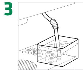
Submerge steam wand in water and heat it up
