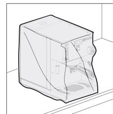
When it has cooled, cover the machine and store it in a dry place, protected from bad weather
