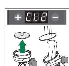
When the display shows CL2, remove the portafilter with blind filter disk and rinse both with water
