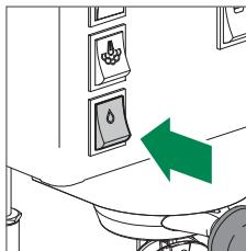
Switch on the hot water switch
