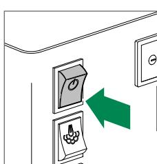
Switch on the machine by shifting the main switch to ON
