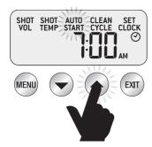
Press UP or DOWN arrow to adjust AUTO START to the desired time (default AUTO START time set at 7:00am).
