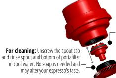
Removable, replaceable spout to enable cleaning and declogging. Each Flex comes with an additional spout. Replace as necessary and if clogged.
