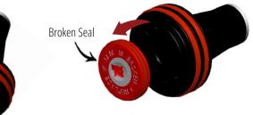
\*Remove the broken valve by pulling it out by the small recess at the edge of the valve. Replace by pushing new valve into the recess on underside of piston, with the foil facing out.
