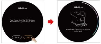
The milk system rapid rinse complete and automatically returns to the main interface
