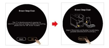
Step 5: Follow the instructions on the screen step by step to perform deep cleaning of the brewing system.
