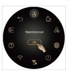
Step 3: Slide the center of the screen to the milk system rapid rinse, click OK;
