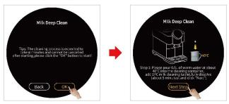
Step 5: Follow the instructions on the screen step by step to perform deep cleaning of the milk system.
