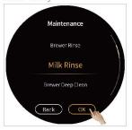
Step 4: Enter the milk rapid rinse, click OK to perform the quick flushing of the milk system.
