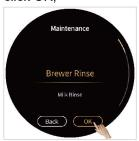
Step 4: Enter the brewer rapid rinse, click OK to perform the quick flushing of the brewing system.
