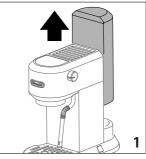
Open the water tank lid (A1) and fill the water tank (A2) with fresh potable water, taking care not to exceed the MAX level (fig. 2).
