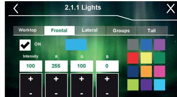
Select ON to switch on front lighting, and choose lighting intensity and RGB colour
