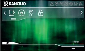
Deactivate screen (the screen will be deactivated for 40 seconds to permit the cleaning)
