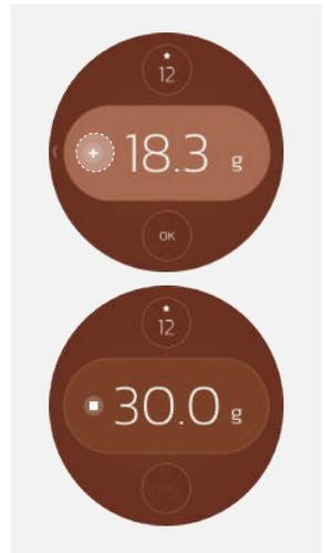
After grinding to the selected weight, press the "+" button to grind more if needed. To stop grinding, tap the "•" button.
